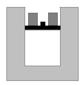
At time **C** we stop adding lead weights to the container and the piston stops moving. The piston is now at exactly the same position it was at time **A**.
