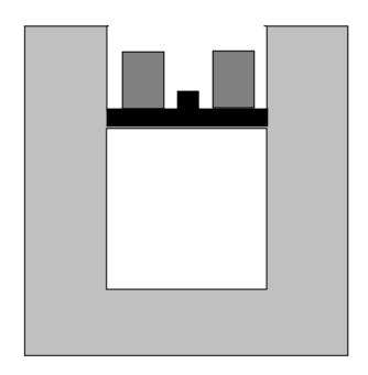
While this happens the temperature of the water is nearly unchanged, and the gas temperature remains practically *constant*.
